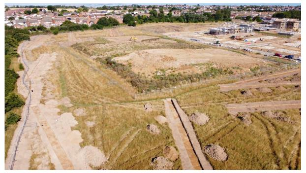
Plate 1 Drone overview of the South and West of site, showing spoil management over area of trenches to be excavated
